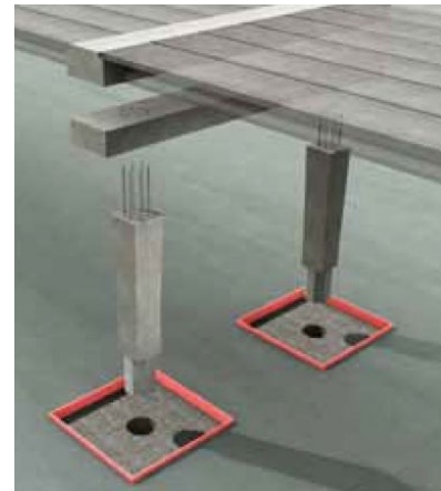
Figure C-120. Integrated Footings and Bent Cap with Columns (Courtesy of PCI Journal, Khaleghi et al. 2012)
